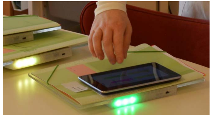
Fig. 1. The Hybrid Patient Record (HyPR) device augments the paper patient record with color configuration and location tracking, while allowing clinicians to pair a tablet which shows the digital information associated with the paper record.
